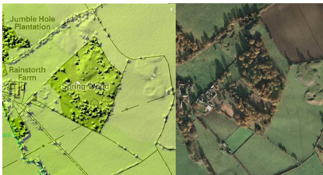
Figure 2: LIDAR Survey has the potential to reveal earthworks (such as these probable bell pit spoil heaps within Spring Wood) that are otherwise poorly visible on vertical aerial photographs.
