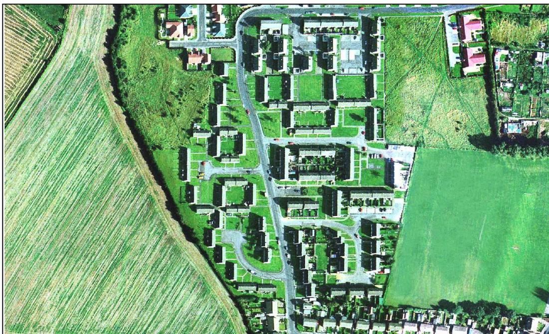
Figure 3: 'Radburn' style estate planning (here in New Edlington) sought to maximise separation of vehicles and pedestrians. Image © 1999 Cities Revealed / The Geoinformation Group.
